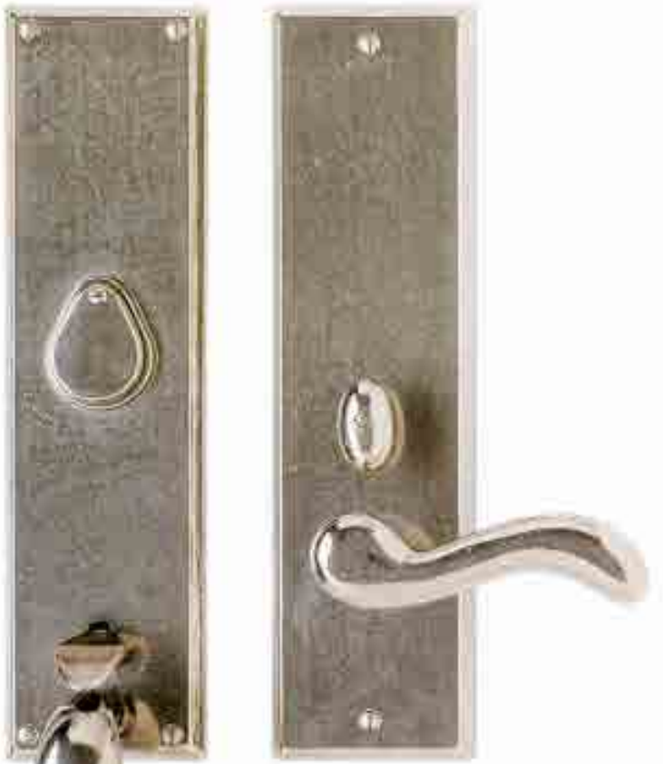
ESCUTCHEONS 3 1/2" x 19 5/8" | 3 1/2" x 13" FUNCTION ENTRY THUMBLATCH MORTISE LOCK GRIP | LEVER G618 6 1/2" COBRA | L112 LARGE CHUB PATINA WHITE BRONZE, LIGHT PART # G542/E463
